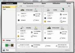
TimberLink F is a tool for monitoring forwarder performance by work stage: Driving empty, loading, driving loaded, and unloading.
